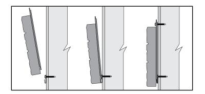
Cut a Beonstone panel and set it in place on the wall. Screw the panel in place. For a **standard framed wall with flexible siding** (gypsum, insulation or bitumen board), be sure to fasten at least one screw in the framing. For **other types of installation**, use two screws per panel, even if the panel has been cut.
