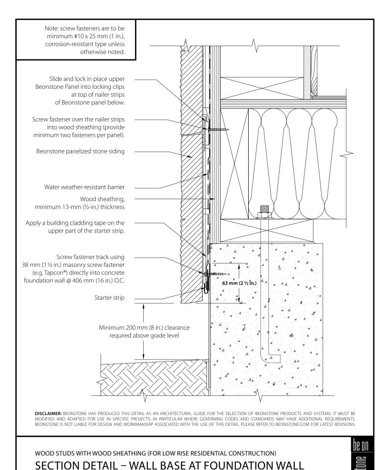
Note: screw fasteners are to be minimum #10 x 25 mm (1 in.), corrosion-resistant type unless otherwise noted.
